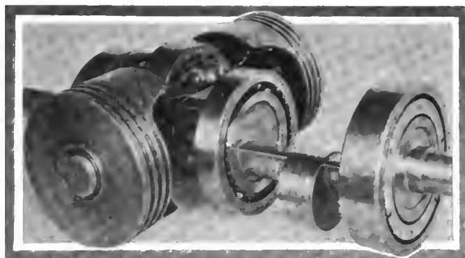
Fig. 6—Crankshaft, pistons and connections between, as used in four-cylinder type of motor
